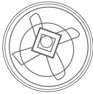
Wrong assemble of blade
